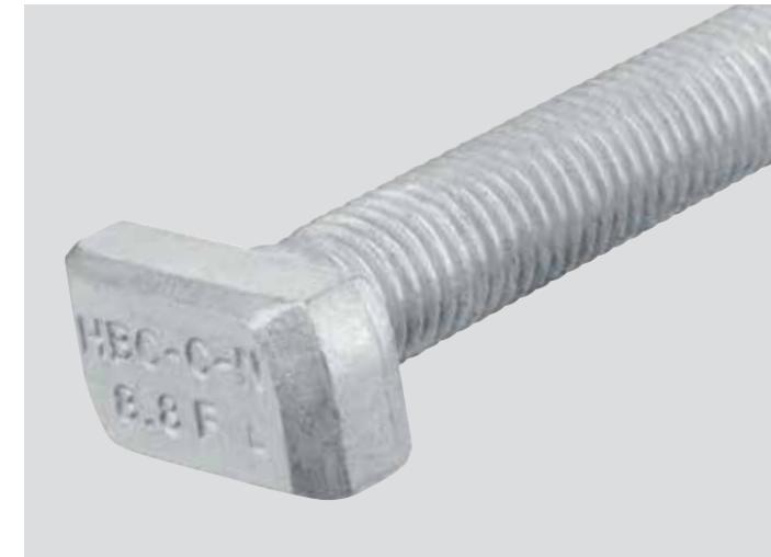
Hilti bolts bear marks on the head indicating the bolt type, strength class, corrosion class and also include a manufacturing mark. The tip of the bolt features a distinct groove that provides a clear indication of bolt head alignment. Bolts with notched heads ("notched bolts") can be identified after installation by the 2 grooves in the tip.
