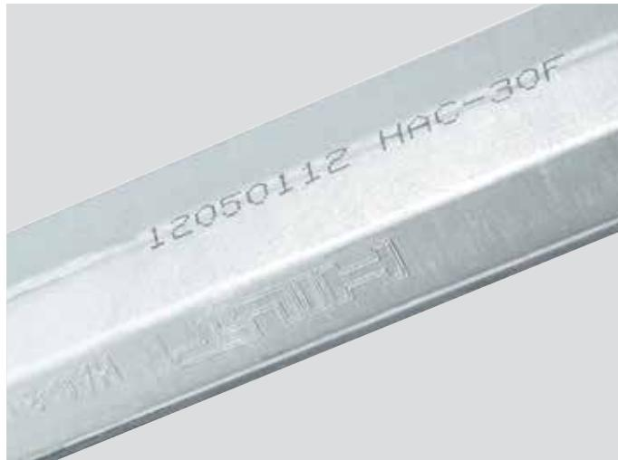
Hilti anchor channels have distinct markings on the outside surface that allow correct identification before casting in concrete. The markings consist of the Hilti logo, the channel type designation and the type of corrosion protection. The channels bear a unique production number that indicates the production lot as well as the channel type, to aid identification.
