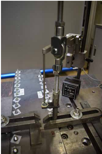
Test set up for tension tests
