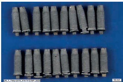
Removed S-BT HL fasteners after 12 weeks EN ISO 16701 cyclic corrosion test. No visible corrosion. No visible corrosion.
