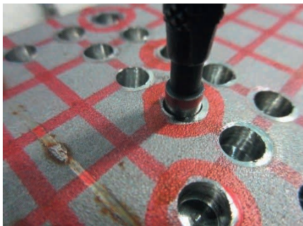
Testing of pilot hole quality
